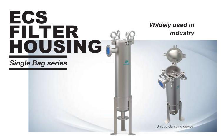
ECS single-bag filter housings with side inlet piping connections and bottom outlet are a perfect choice for cost-sensitive applications. The side inlet piping connections can be adapted to different directions, according to your specific needs. The simple design allows an easy cleaning of the interior. Precision castings and swing eye-bolt closure guarantees integrity even at high pressures.
